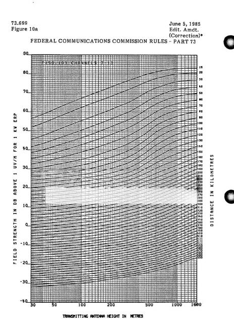
ESTIMATED RELD STRENGTH EXCEEDED AT 60 PERCENT FCC 73.699 Figure 10a OF THE POTENTIAL RECEIVER LOCATIONS FOR AT LEAST 50 PERCENT 10 PERCENT\* OF THE TIME AT A RECEIVING ANTENNA HEIGHT OF & METERS
