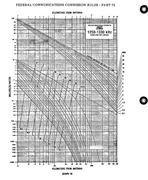
The curves are labeled with the ground conductivities in millisiemens/meter. All curves except the 5000 mS/m (Sea Water) curve are derived for a relative dielectric constant of 15. The sea water curve is derived for a dielectric constant of 80.
