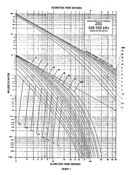
The curves are labeled with the ground conductivities in millisiemens/meter. All curves except the 5000 mS/m (Sea Water) curve are derived for a relative dielectric constant of 15. The sea water curve is derived for a dielectric constant of 80. FCC/73-140 -107 -
