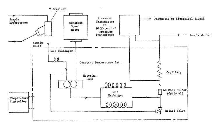
Figure 1 — Schematic Flow Diagram
