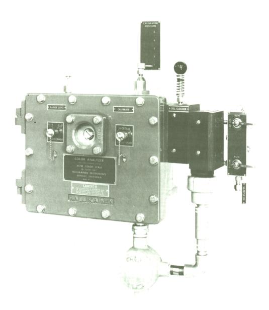
The COLOR ANALYZER is a differential photoelectric colorimeter providing an output signal for recording color determination of petroleum products or other liquids within the limits of measurement of the instrument. A unique feature includes the use of ASTM glass color standards for calibration purposes. These glasses are the same as those used in the petroleum industry for visual comparison tests described in the ASTM-D-1500T method.
